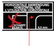
Also authorised for horizontal application in case of Edge radius  $r = 0.5$  mm without burr, where the angle of the edge implementation must be at least 90° degrees.
