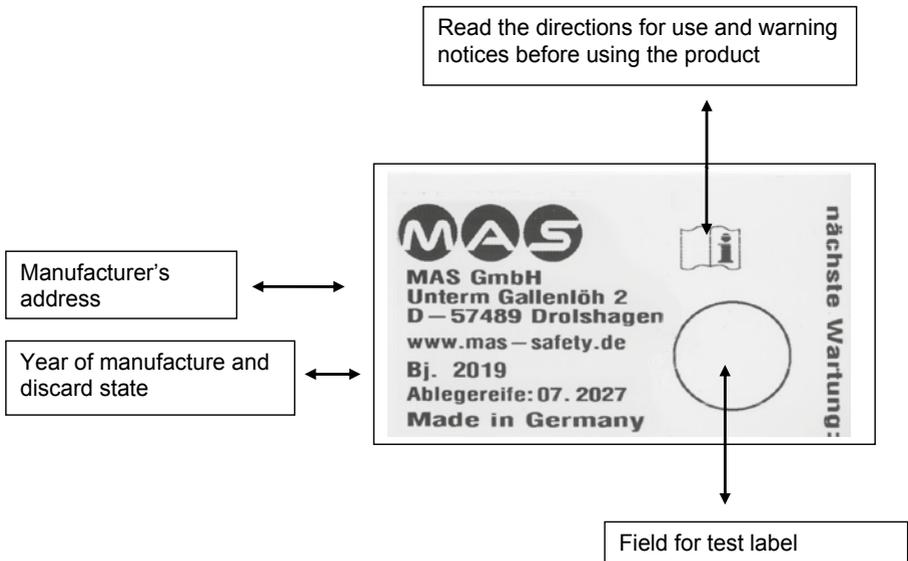
**A** → Labelling of the harness eyelet on the harness belt
